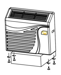
Step 1: Lift up the dehumidifier and let it sit on the wooden box as show on figure below.
