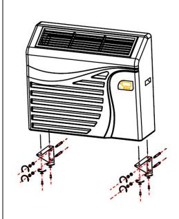
Step 1: Choose the right installation position for the wall support according to the size of installing holes and the wall bracket holes position. The installation position should guarantee the dehumidifier in horizontal position. The position of the exploded screw should be marked.
